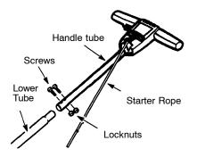
NOTE: When performing the following step, be sure the starter rope is not caught under the cable clamp. The starter rope must hang freely to operate properly.
